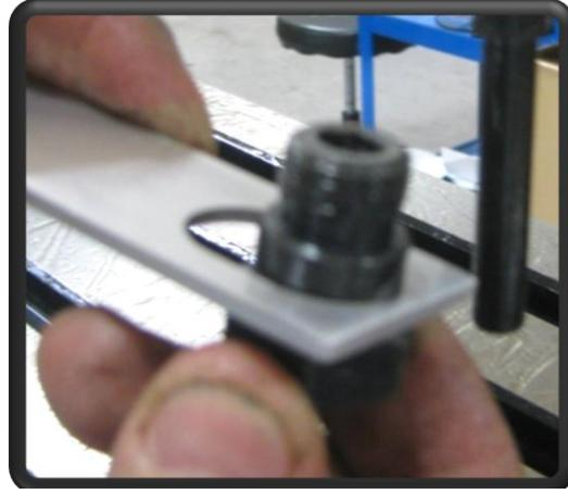
7. Adjust the position of the limit switch bracket so that it triggers the switch against the strike plate just before the top limit of Z travel.
