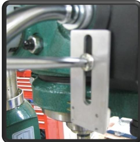
6. Loosen the two set screws on the side of the Z travel adjustment knob and remove the knob. Place the Z+ strike plate on the knob as shown, replace the knob back in its original position and tighten the set screws.
