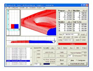
Includes FlashCut's intuitive Windows based CNC software that can be easily tailored to control any machine tool.
