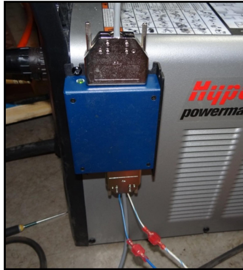
Example of THC Isolation Box Mounted to the Torch
