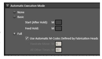
**Start (After Hold)** FlashCut can execute an M-Code whenever **Start** is clicked after a feed hold has occurred (but not when initially starting the file).
