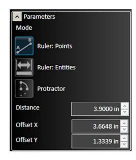
Ruler used to measure between the distance between points: center of an arc, and radius of an arc. Note the construction lines marking the other sides of the triangle: these represent the **Offset X** and **Offset Y**
