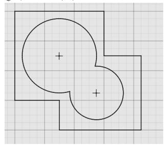
The results of a **Weld Cutouts** operasion
