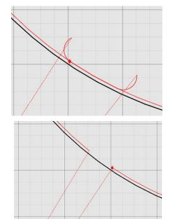
In the examples to the right, the top drawing shows a closed break with an overburn. The cut begins with an arc-shaped lead in, and finishes with an arc-shaped lead out. The parameters for this break are shown below.
