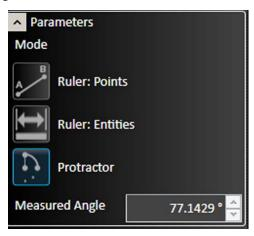
**Protractor** used to measure the arc and **Measured Angle** between two points of a polygon. Note that the protractor will not measure an arc or angle if it is grouped with other lines or shapes. You must ungroup the arc to enable the protractor tool.
