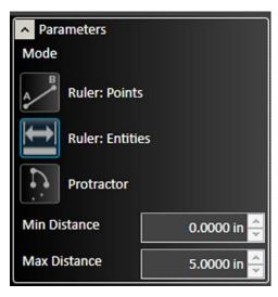
Ruler used to measure the distance between two entities: adjacent sides of a rectangle. Note that the **Min Distance** and **Max Distance** appear on the drawing, as do the lengths of the two sides.
