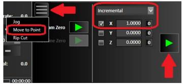
3) If the motor stalls, decrease the Start/Stop Feedrate and repeat the motion. If the motor doesn't stall, increase the parameter and repeat.
