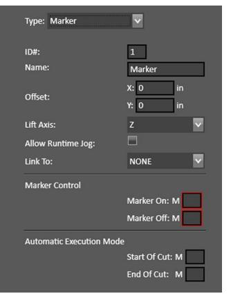
**Start/End of Cut** – Enter the Automatic M-Codes or Macros for turning the marker on for cuts and off for rapid movements. Note that the Macros and M-Codes must be defined in the M-Code Definitions. Automatic Execution must be enabled in M-Code Execution.
