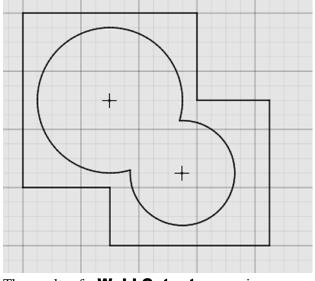
The results of a Weld Cutouts operasion
