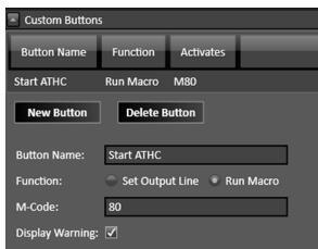
Custom buttons appear in the CNC window. They are located in a panel to the left of the drawing workspace.
