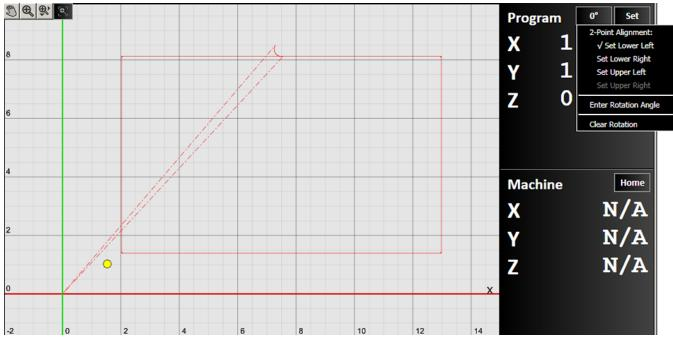
5. Jog the tool position to the lower right corner of the workpiece
