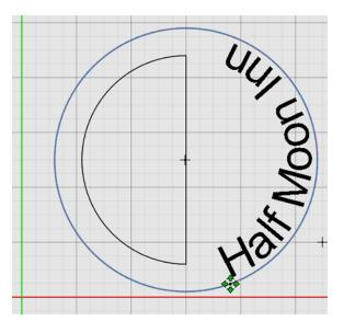
The resulting CAM toolpath for the sample drawing appears below. Note that it is not necessary to explode letter shapes to create toolpaths.
