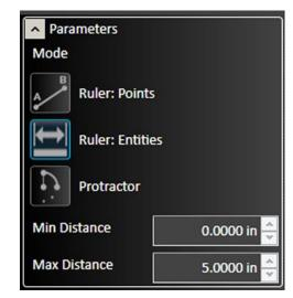
Ruler used to measure the distance between two entities: adjacent sides of a rectangle. Note that the **Min Distance** and **Max Distance** appear on the drawing, as do the lengths of the two sides.
