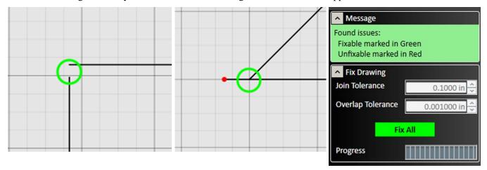
Use the **Search Issues** button to identify issues with the drawing that could lead to mistakes in fabrication. Issues noted with a green circle can be fixed automatically by selecting **Fix All**. Issues noted with a red circle must be addressed manually.
