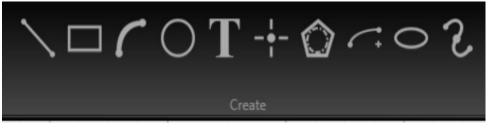
You may use the mouse to place and size each element or you can edit parameters for the element, such as dimensions and location, in the parameter window after creating the element. Click the shape or features and then edit the desired parameters.
